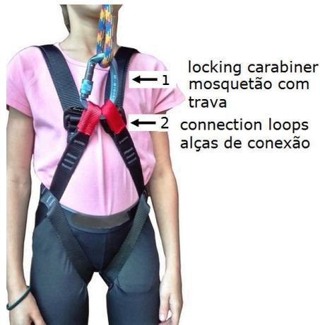
**FIGURA 2:** properly dressed harness. Both red connection loops must be clipped with the carabiner. Position the carabiner in a way that the locking barrel locks going down. In that way, any trepidation during the use helps to lock the carabiner, instead of unlocking it. Also, the rope can be tied straight to both connection loops using a follow through figure eight knot.
