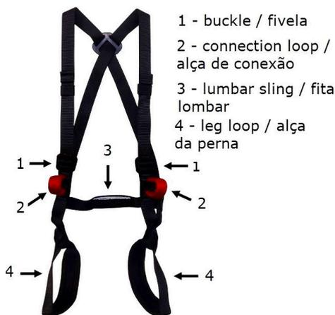
**FIGURA 1:** Zion harness and its parts. Red connections loops should be in front and lumbar sling on the lower back of the user.
